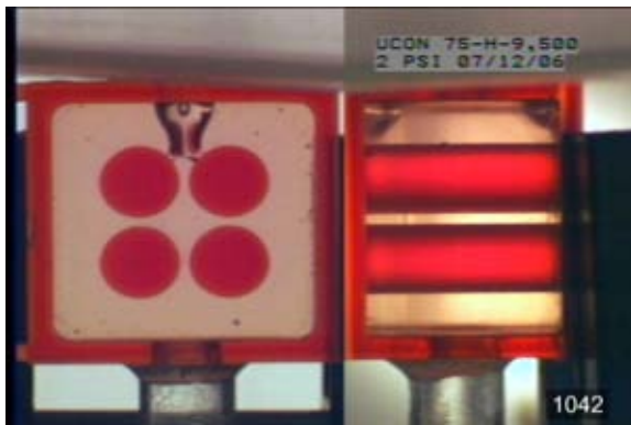
Figure 37. 3D ARIA calculation correctly shows bubbles left at exit near walls. Left, views of the experiment (left from front, right from side) as liquid knit lines meet and as liquid begins to leave the top. Right, corresponding frames from simulation.
