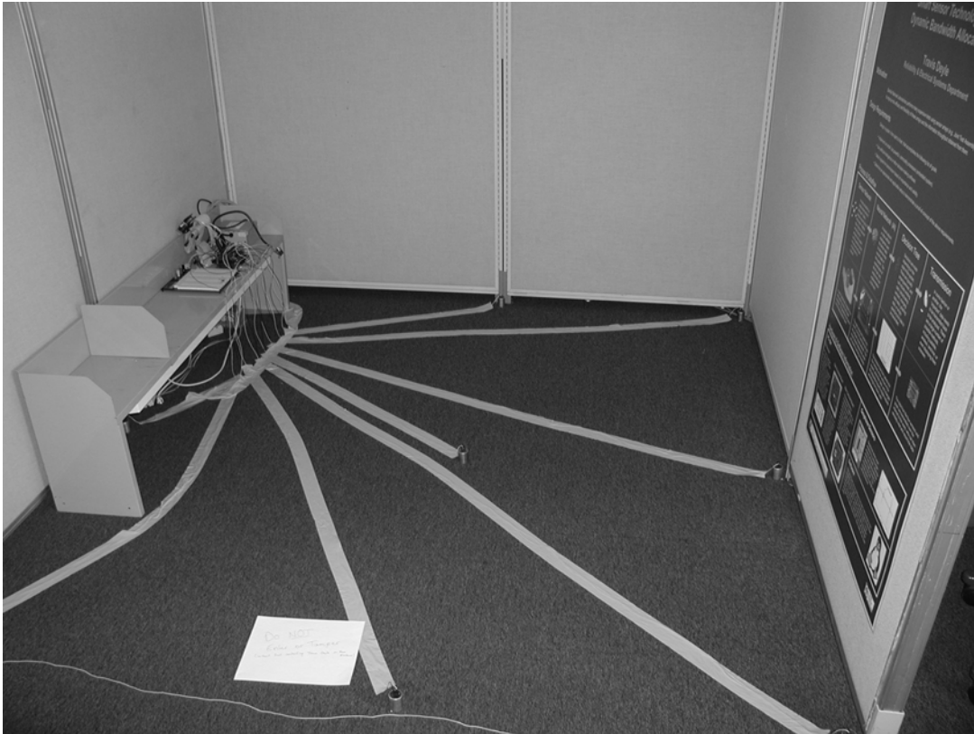
Figure 9. Geophone sensor array. The geophones are laid out in a 3 x 3 grid.
