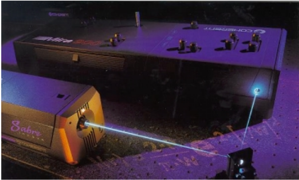
Figure 2.1: Femtosecond laser system used in teleportation experiments
