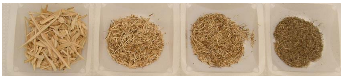
Figure 1: Photographs of fractionated dryer fines. The samples from left to right correspond to ID1-4, respectively, in Table 1.
