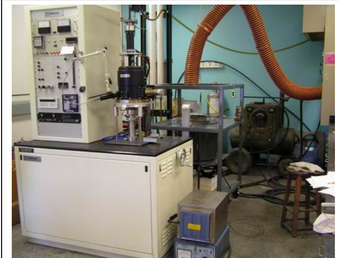
Figure 3.2 Microwave assisted electrolytic cell system
