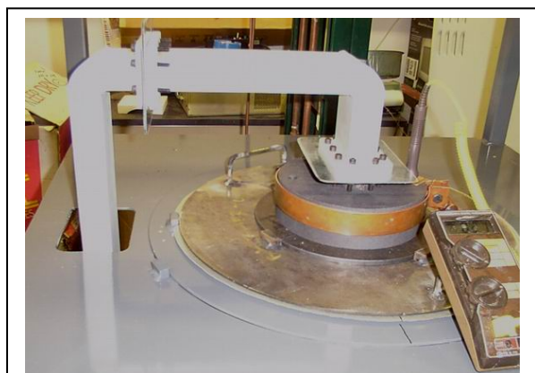
Figure 3.5 Waveguide and graphite anode
