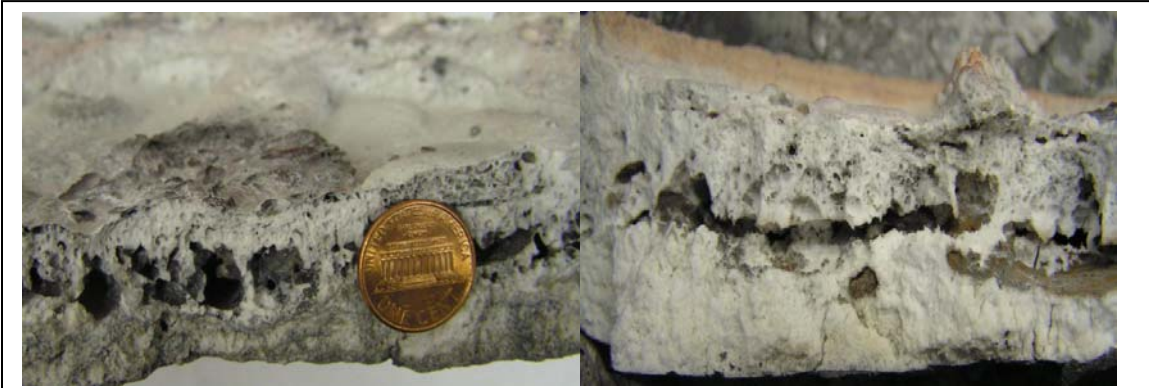
Figure 4.4 Multi-layer structures of solidified slags (with microwave irradiation) (Left): lower section shows gray color in one slag; (Right): lower section is white but denser in another slag.
