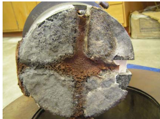
Figure 4.40 Fluoride in graphite channel with microwave irradiation
