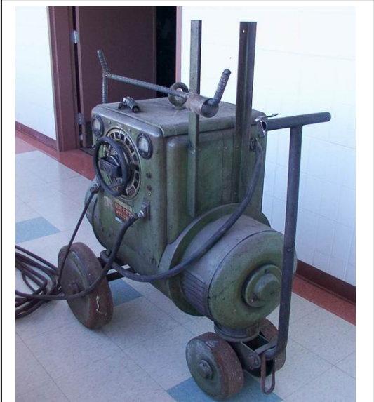
Figure 3.11 Direct current supplier, providing DC up to 200A
