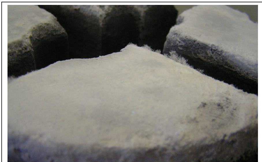
Figure 4.5 Dendrites on the bottom surface of graphite anode
