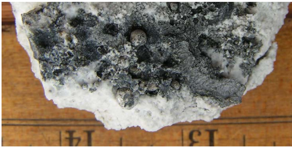
Figure 4.11 Aluminum beads contacted graphite lining
