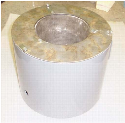
Figure 3.6 Electrolyte bath (cathode made of a nickel-based superalloy, working up to 1200°C)
