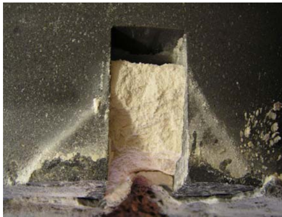
Figure 4.39 Fluoride in graphite channel without microwave irradiation
