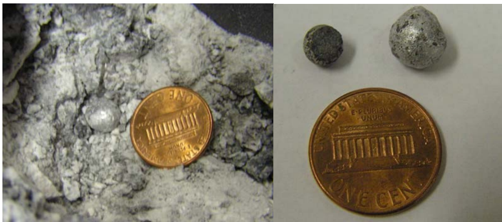
Figure 4.12 Size of the aluminum beads increased with microwave irradiation (the largest aluminum bead: about 10mm in diameter)
