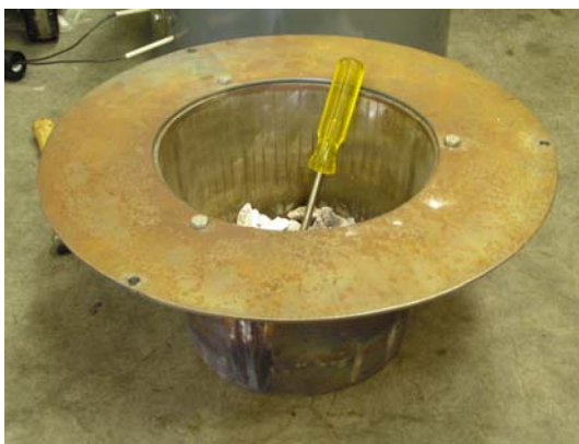
Figure 3.8 Nickel-based superalloy bath
