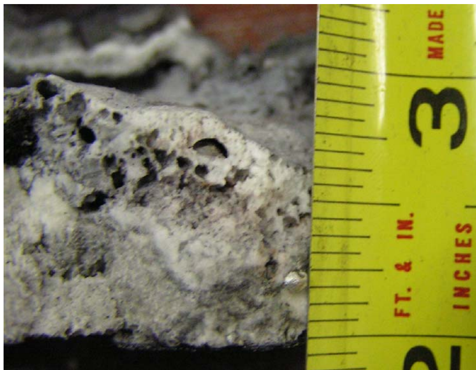
Figure 4.10 Aluminum beads in the porous layer
