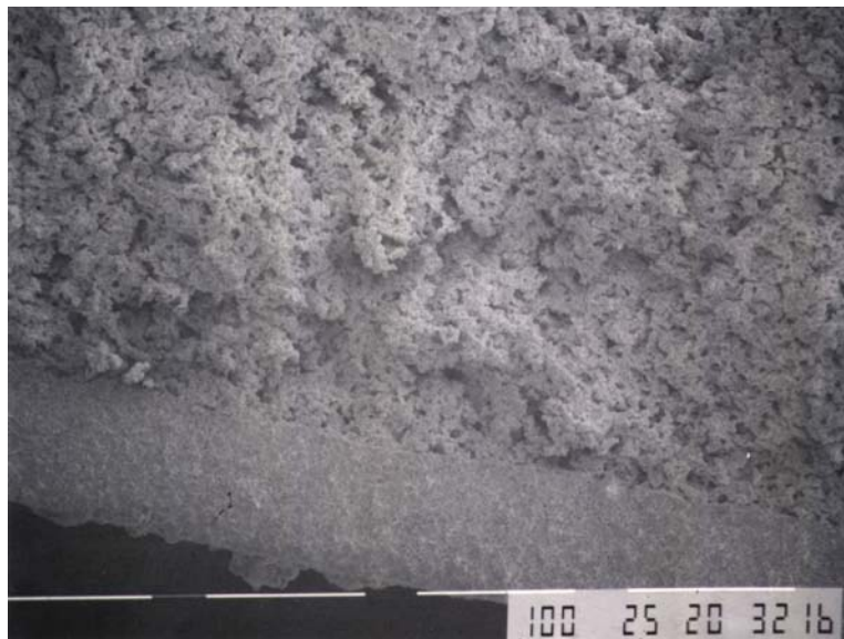
Figure 88. SEM image of a dense thin ceramic film (bottom) on a porous support of the same composition (top). The white bar represents 100 \mu\text{m} , which is also about the thickness of the film.
