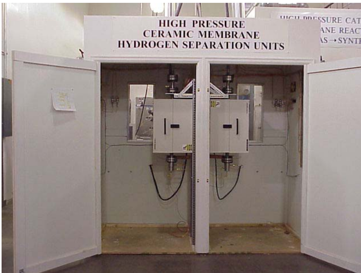
Figure 74. Photograph of the apparatus for evaluation of hydrogen separation membranes at high pressure.
