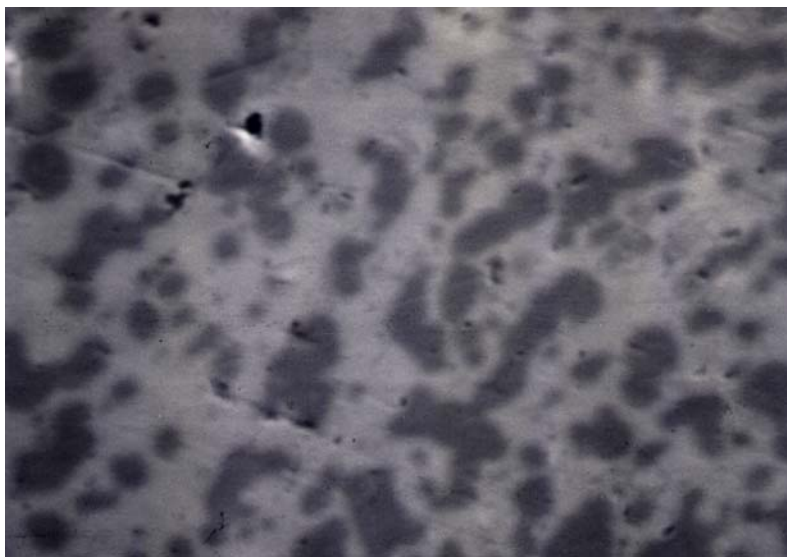
Figure 26. SEM image of a 56/44 wt.% ceramic/metal membrane. The dark regions are the metal phase and the light regions are the proton conducting ceramic.
