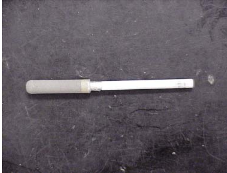
Figure 93. Dense BCY/Ni thin film tube brazed onto a 1/4" alumina tube.
