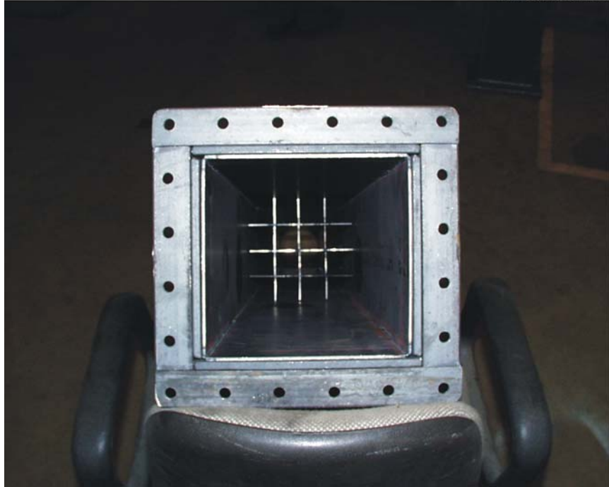
Figure 9. Flow straightener inside of reactor chamber.
