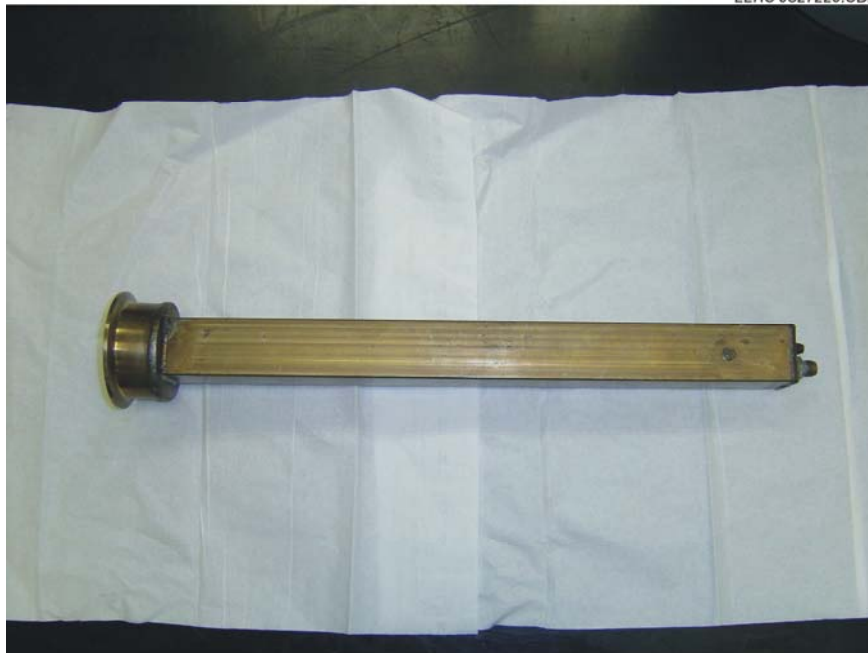
Figure 13. Catalyst holder for bench-scale testing. The rectangular section is approximately 14 inches long.
