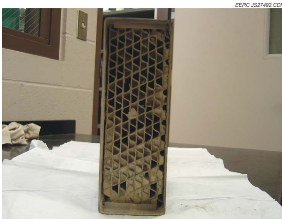
Figure 23. Catalyst section removed after 43 days of operation.
