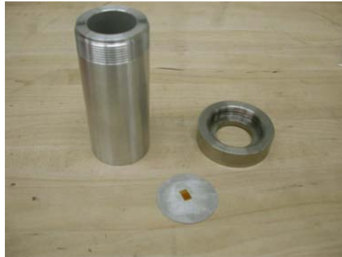
Fig. 8: Test geometry used for assessing the mold releasing performance of six different products.
