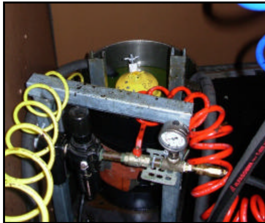
Figure 4. Close up of Oil Bath and Centrifuge.
