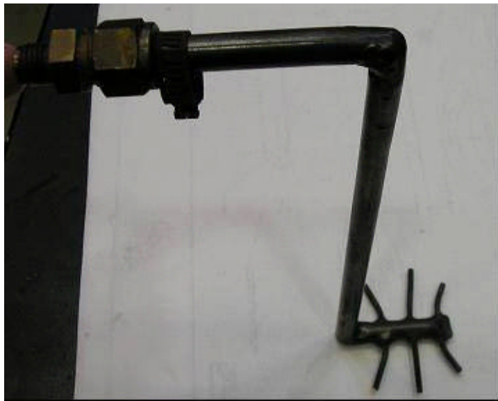
Figure 43. Photograph of Sparger Used for Bubbling Air Along the Cathode.
