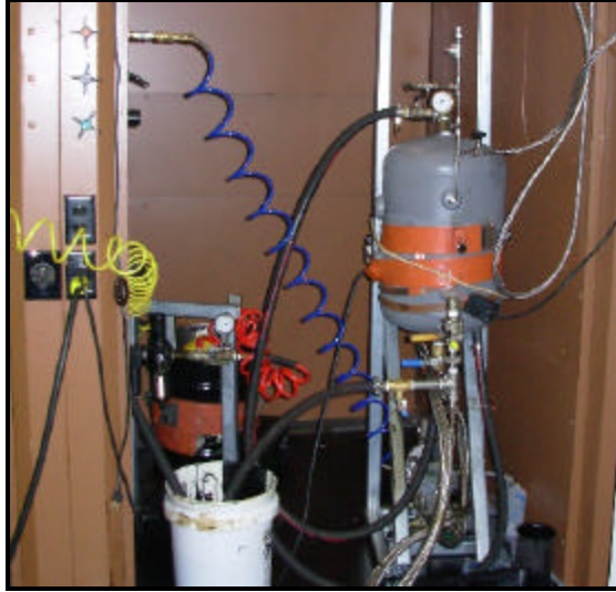
Figure 3. Centrifugation system, showing pressurized holding tank and centrifuge.
