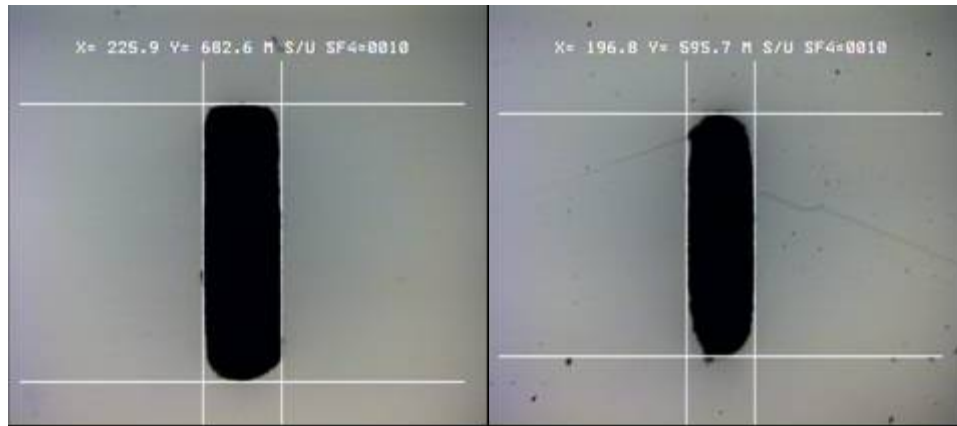
Figure 2-4. Pyrex shadow mask. Top shown in left figure, bottom shown in right figure.
