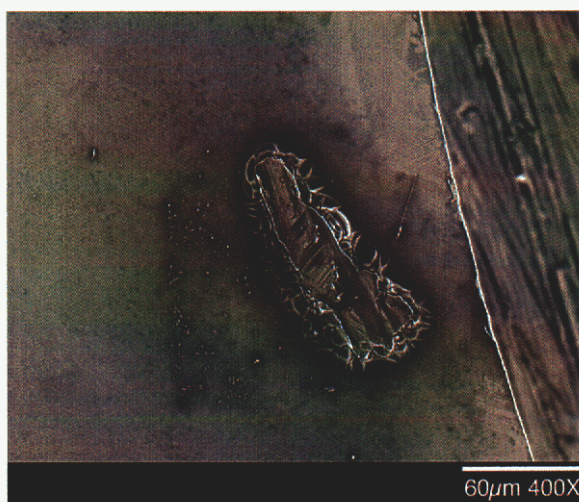
Figure 37. Flakes of material embedded in the release side of tensile bar 1041; these flakes are thought to be steel since EDS reveals that they are rich in Fe and Cr.
