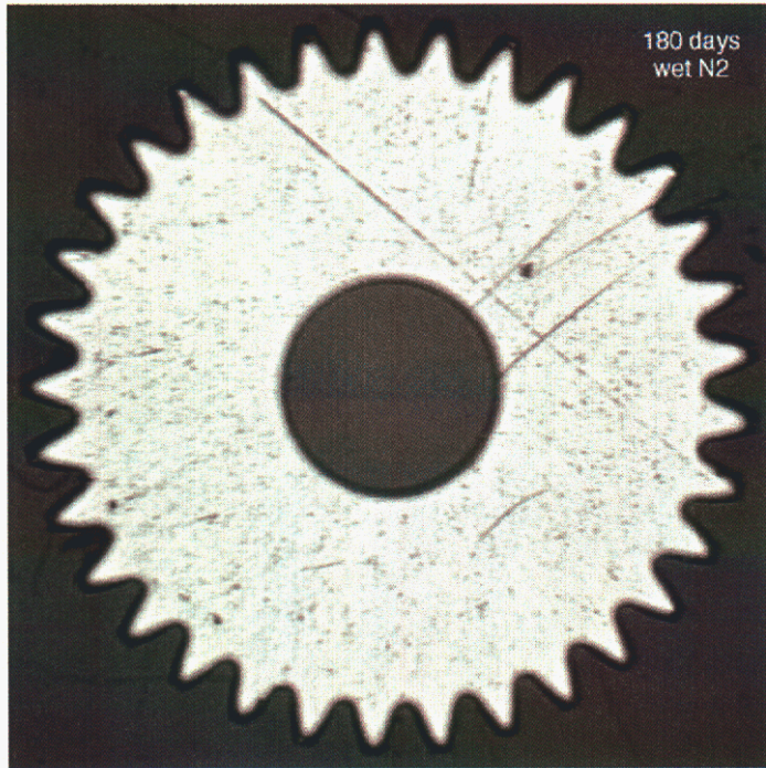
Figure 35. Images before and after dormancy for (a) washer 2015, (b) gear 3014, and (c) u-spring 4014.
