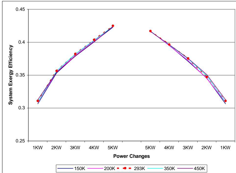
System Energy Efficiency for perturbations of inlet Steam temperature for power increases and decreases
