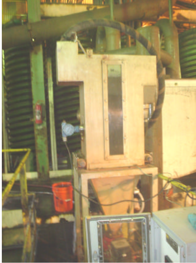
Figure 1.18. The 9x16-inch Pilot-Scale CrossFlow Separator Test Circuit at Plant E.
