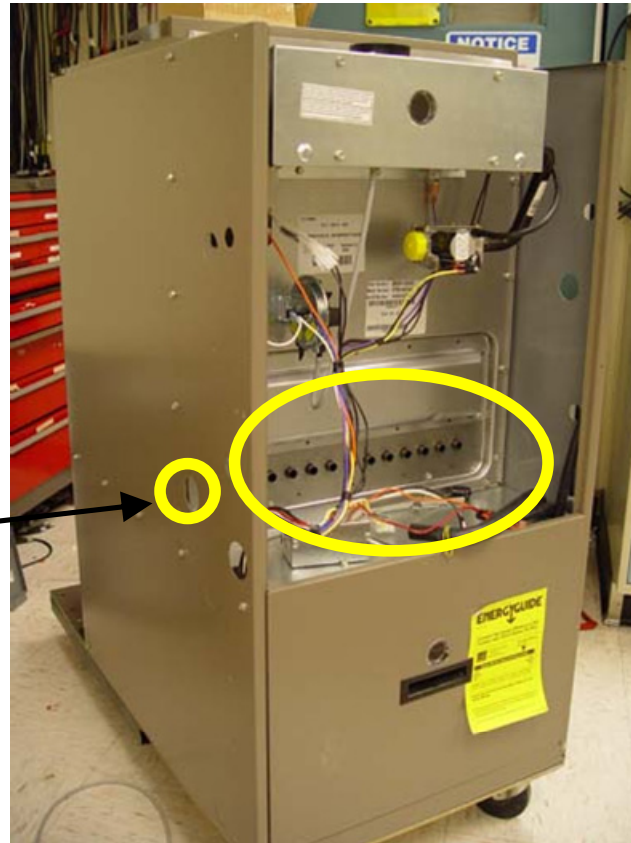
Figure 4: Photograph of modifications made to a residential furnace that allows installation of the spectrometer.
