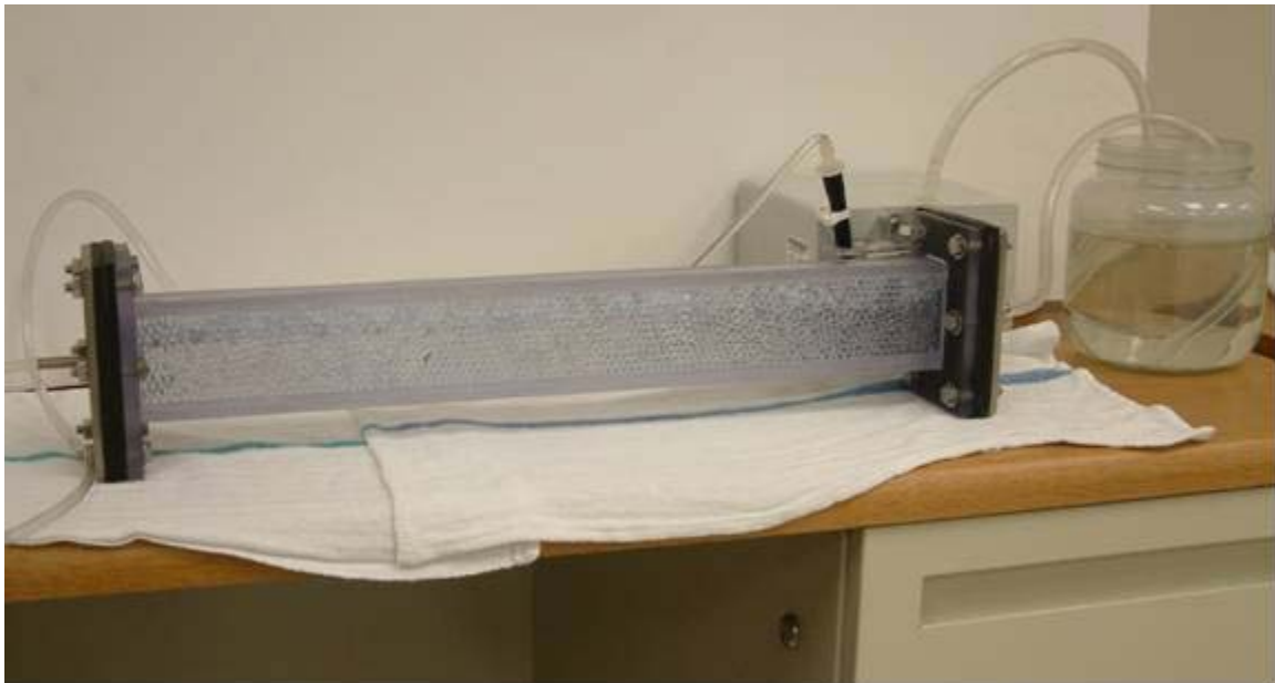
Figure 6. Modified Hele-Shaw Cell Packed with 5mm-glass beads
