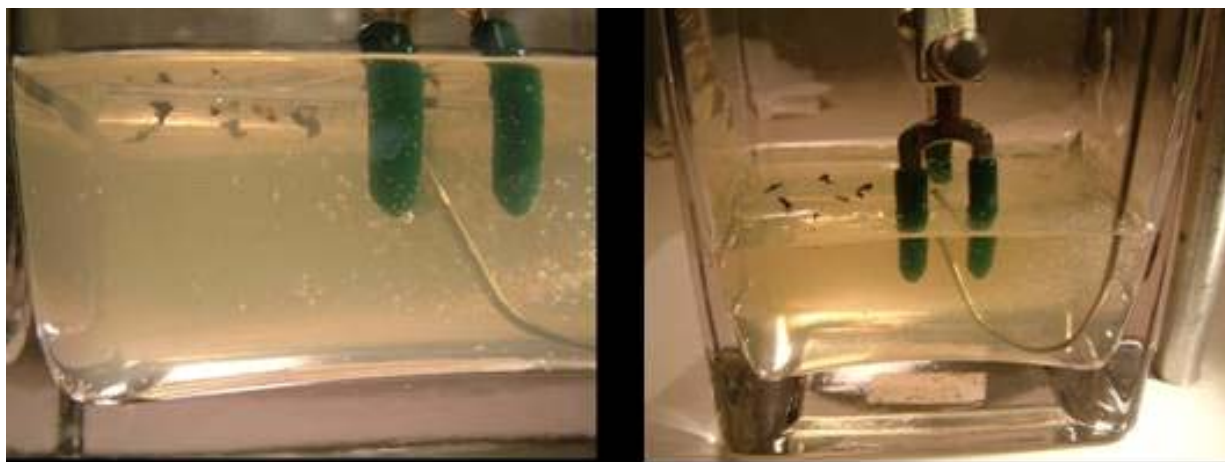
Figure 8: Sessile Drop Apparatus: Dark Oil and Transparent APHRON ICS™ Mud
