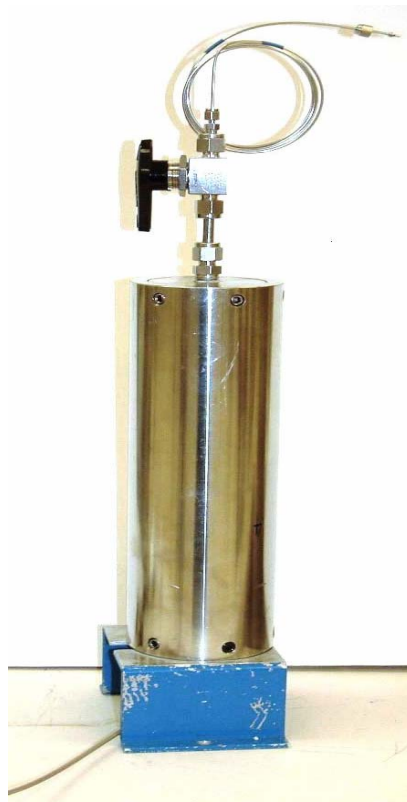
Figure 14. Capillary Flow Test Apparatus
