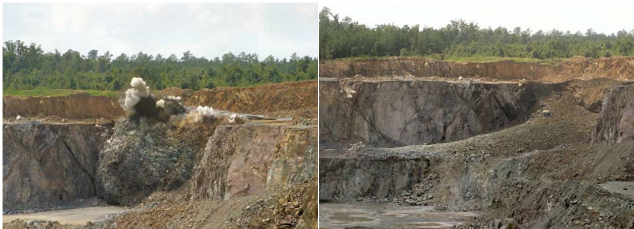
Figure 12. Photograph of blast 8605 soon after initiation clearly showing minimal stemming region and good face movement; second photo shows muckpile.
