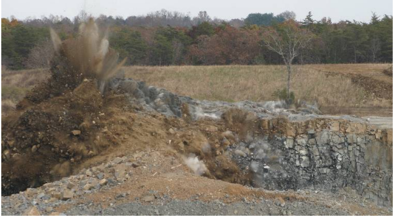
Figure 22. Photograph of the LS blast clearly showing oversized blocks in the free face.
