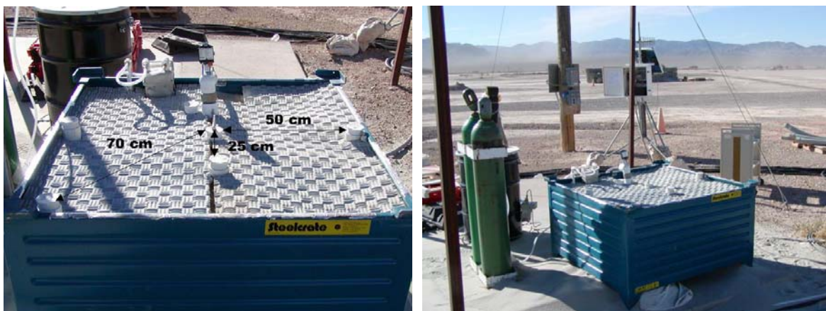
Figure 70. Sandbox Test. Left: Placement of tubes for contaminant (center tube) and sensors. Right: Sandbox with data-logging station in background. (from Ho et al., 2002)
