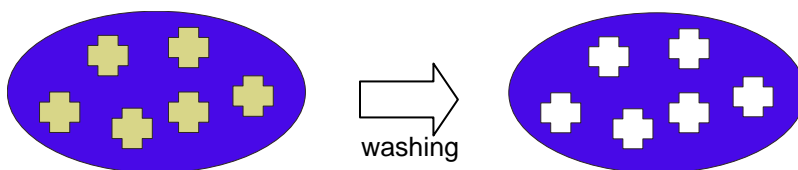
Figure 78. Illustration of molecular imprinting by polymerizing monomers around a target biomolecule (e.g., bovine serum albumin). The left images show the target biomolecules mixed with the polymer matrix. The right image shows the polymer structure after the biomolecules have been washed out, leaving behind an imprint (or hollow regions) in the polymer. These imprints provide a geometrically specific site for the target biomolecule to rebind into.
