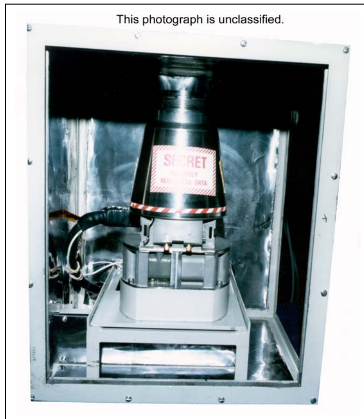
Figure 1: AF&F unit mounted in its cassette for active testing in the Middle Note event, 18 March 1987. The apparent left-to-right “key holing” of the cassette is an artifact of the photography. (Courtesy of Frank Dean.)
