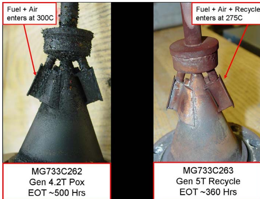
Figure 5.3.7.2-1 - EOT NG1 Mixing Cone
