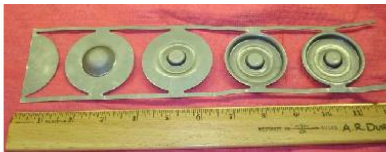
Figure 5.3.1.2.2.4.1-1 - H230 Stamped Samples Using Available Tooling
