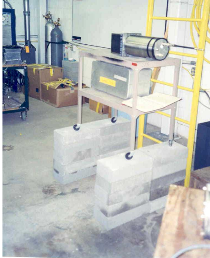
Figure 16. Layer Cake placed on thin metal table (to minimize neutron scattering) on stacked cinderblocks; at this height the detector was aligned to center of DPF
