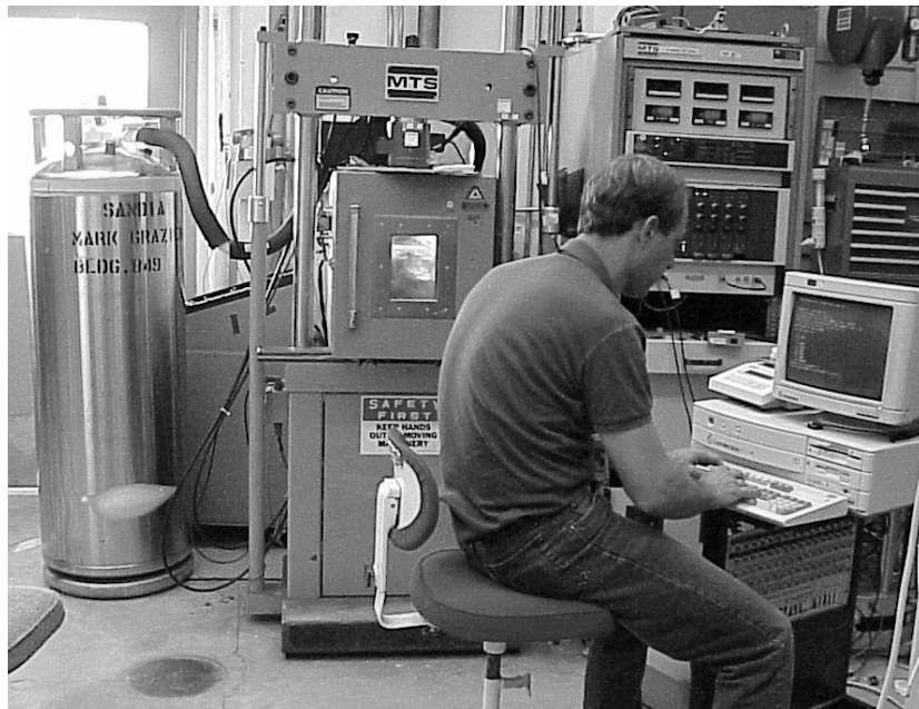
Figure 12. A uniaxial compression test set-up consisting of a 0.1 MN load-frame and an environmental chamber for temperature control.
