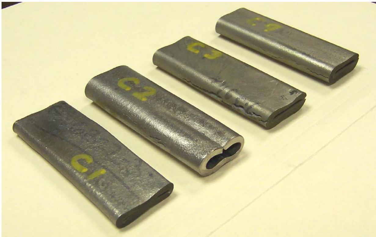
Figure 4.9: Crush test samples after the test, Sample C1 (left) did not crack. Samples C2, C3, and C4 (right) cracked.
