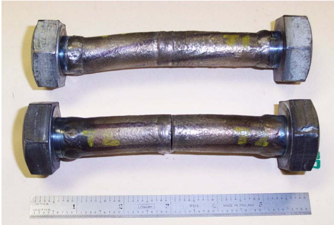
Figure 4.1: Torsion test sample after test (T1 top, T2 bottom)
