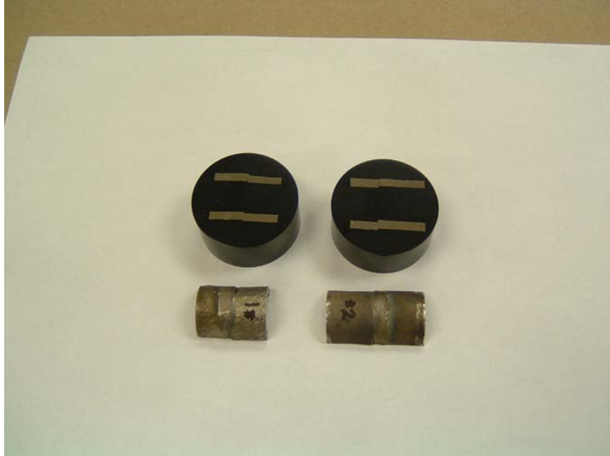
A. A view of the samples containing the brazed joints (taken following sectioning and mounting).
