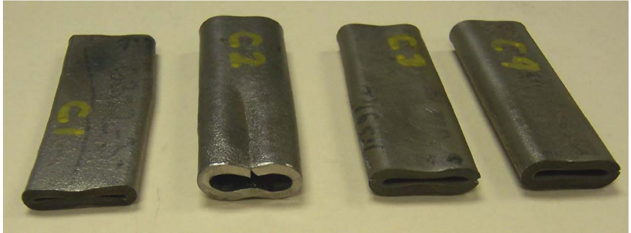
Figure 4.8: Crush test samples after the test, Sample C1 (left) did not crack. Samples C2, C3, and C4 (right) cracked.
