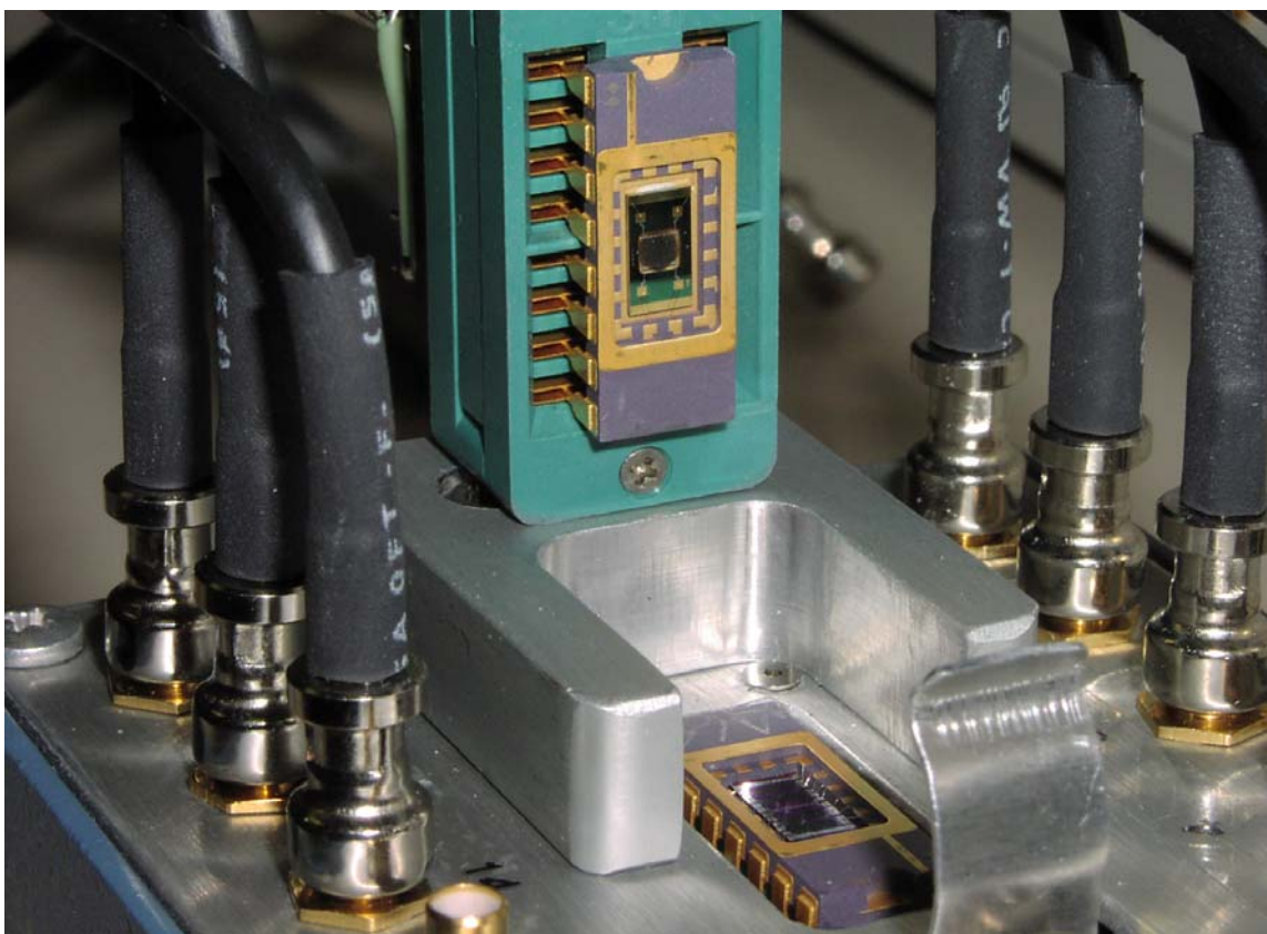
Figure 2: Chemiresistor and preconcentrator dies with custom housing for face-to-face mating. Both the chemiresistor die and preconcentrator die are packaged individually in 16-pin DIPs. The custom housing allows face-to-face mating and a decreased diffusional path length compared to the planar lateral arrangement in a single DIP. Decreased diffusional path length is anticipated to translate directly to more efficient transfer of preconcentrated analyte from the preconcentrator to the chemiresistor sensor, and hence greater response from the sensor and lower detection limits.
