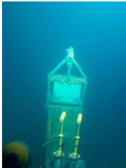
Picture 1. The PFA (pore-fluid array) which had been deployed in May, 2005 was located upright with its probe inserted into the sediments.
