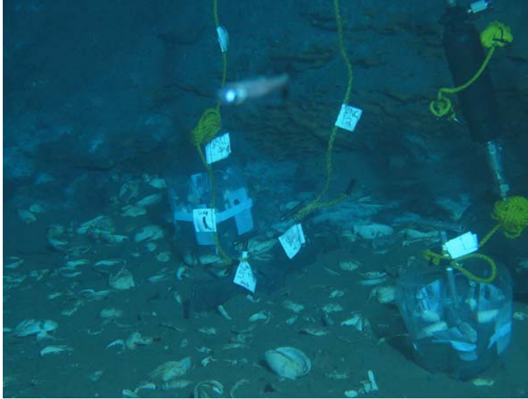
Picture 6. Four Pore-water equilibration devices (peepers) were placed along a transect away from a wall containing gas hydrate to determine methane concentration gradients.
