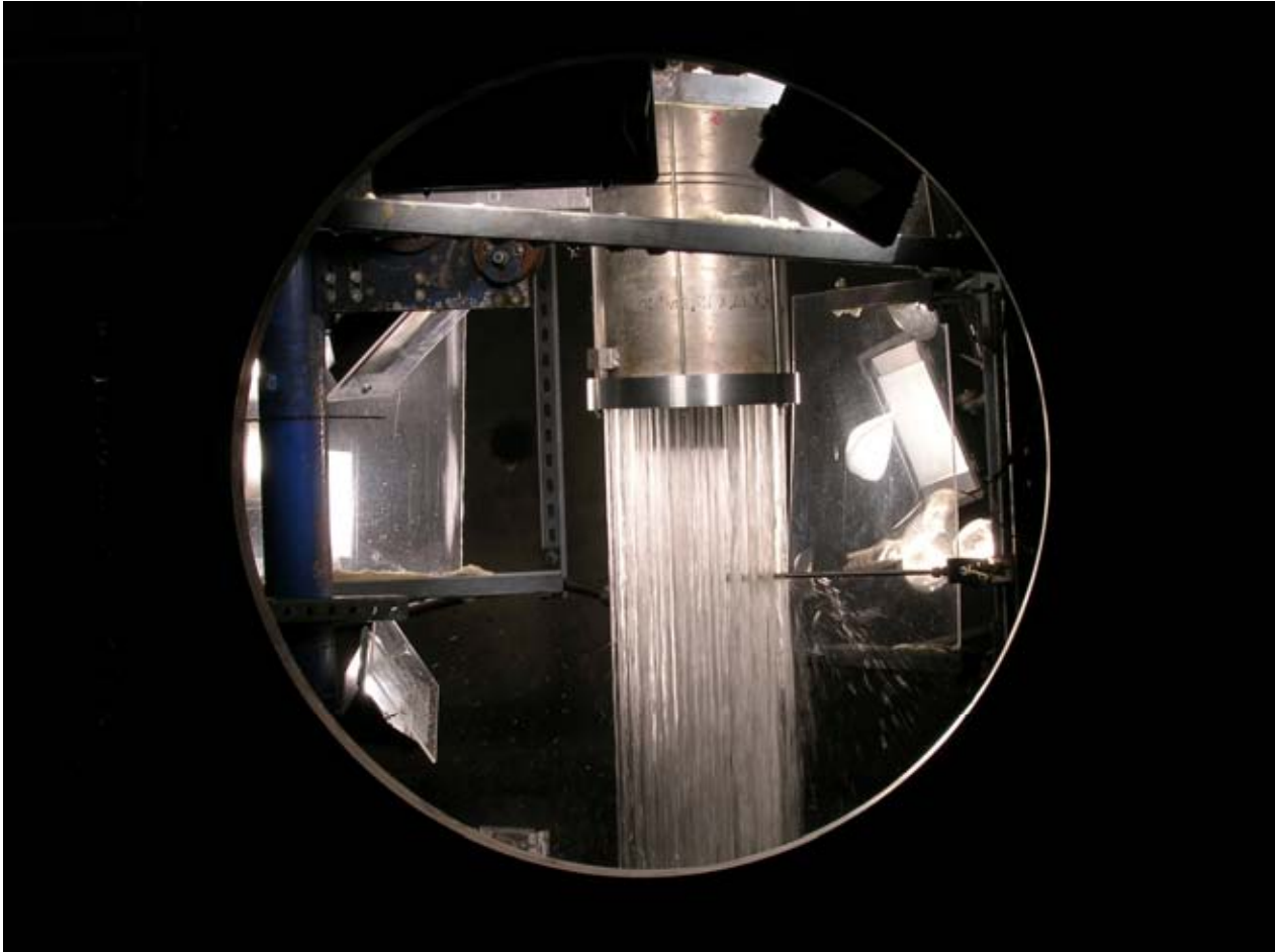
Figure 4.16: Phase 2 nozzle in operation inside the VHEX chamber. Horizontal rod entering from left supports the explosive charge located on a stalk centered in the array 10 cm above the rod.
