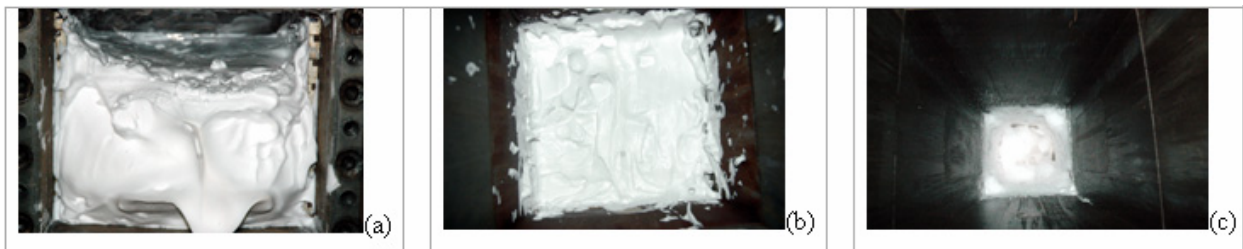
Figure 4.41: Shaving cream foam photographs in shock tube, (a) side-view during fill, (b) top view pre-test, and (c) top view post test
