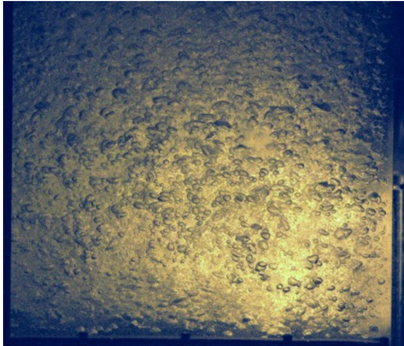
Figure 4.37: Water with 15% void fraction of Ar in a mock-up of the shock tube test section with transparent walls- the width of the test section is 25.4 cm.
