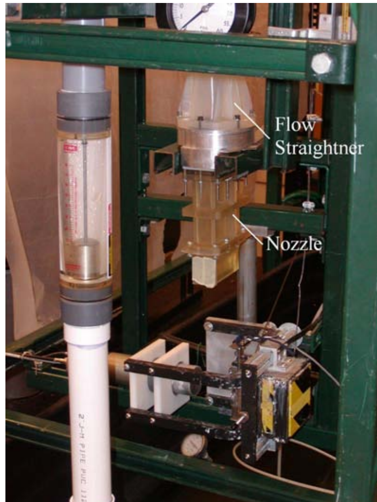
Figure 4.22: Experimental setup highlighting the flow conditioner and nozzle.
