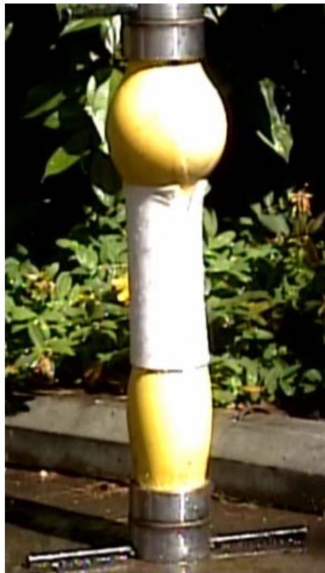
Figure 41: Quick burst test with overlapping full-wrap gel film patch shows successful bond at 500 psi
