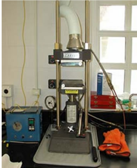
Figure 19: Carver press equipped with heated platens
