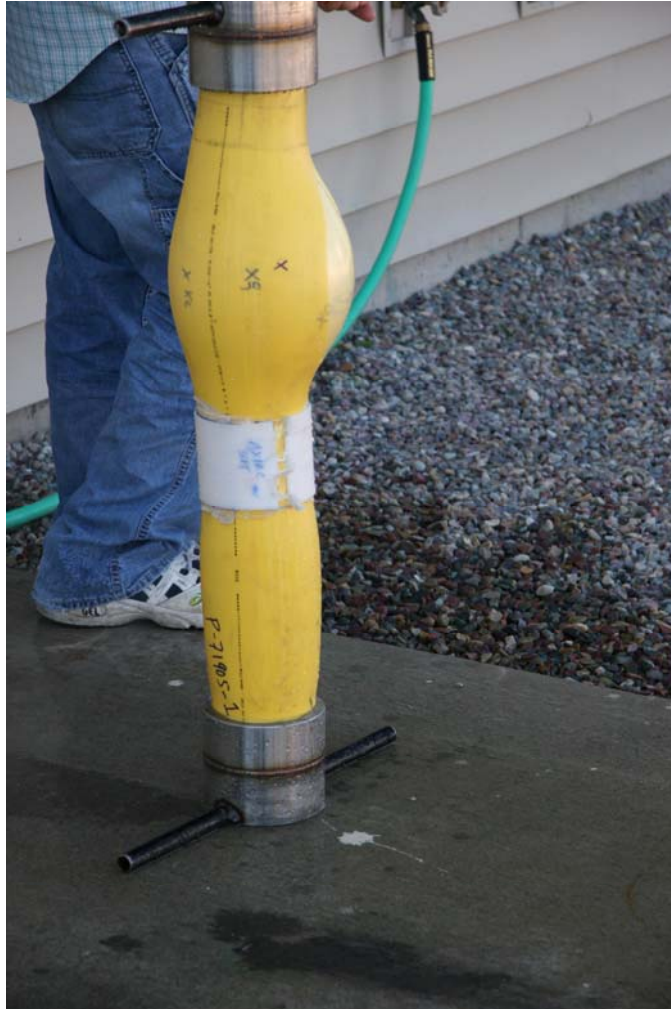
Figure 31: Quick burst test for DOE/NETL demonstrates successful bonding of PE gel film patch on 4-inch MDPE pipe
