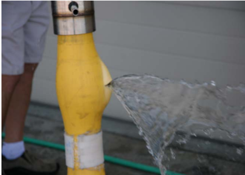
Figure 24: Successful bond of PE gel patch to 4" MDPE pipe at 600 psi during quick burst testing
