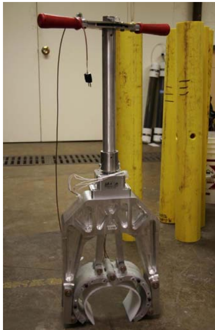
Figure 13: Final Test Tool with Repair Patch
