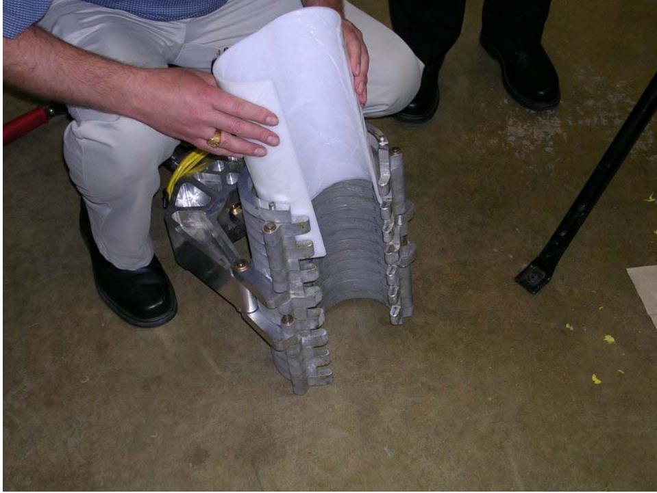
Figure 48: PE gel film repair patch being loaded into the engineered prototype for Nicor Gas demonstration in Naperville, IL
