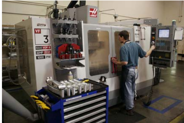
Figure 12: Computer Numerically Controlled (CNC) Machining Center
