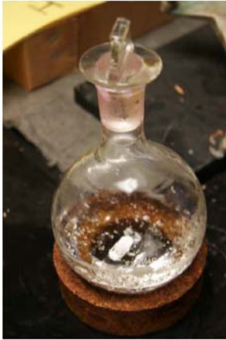
Figure 15: UHMWPE powder dissolved in heated solvent
