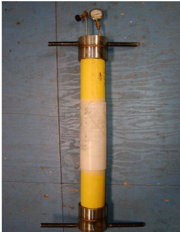
Figure 43: Closed system overlapping full-wrap gel film patch held at room temperature & 200 psi for > 5 months without any loss in pressure
