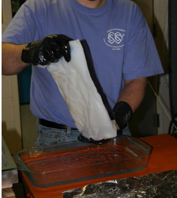
Figure 38: Photo of the final large PE gel film patch after the swelling process
