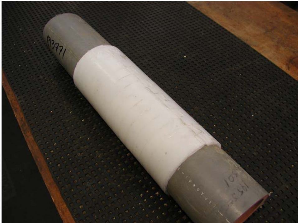
Figure 51: Overlapping full-wrap PE gel film patch successfully bonded to oxidized 4-inch IPS Aldyl-A pipe during demonstration for Sempra Energy
