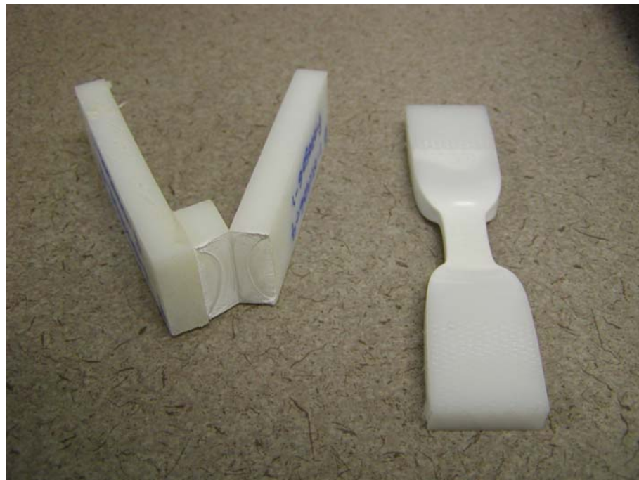
Figure 47: Broken embrittled HDPE material (left) compared to typical necking in HDPE control sample (right)
