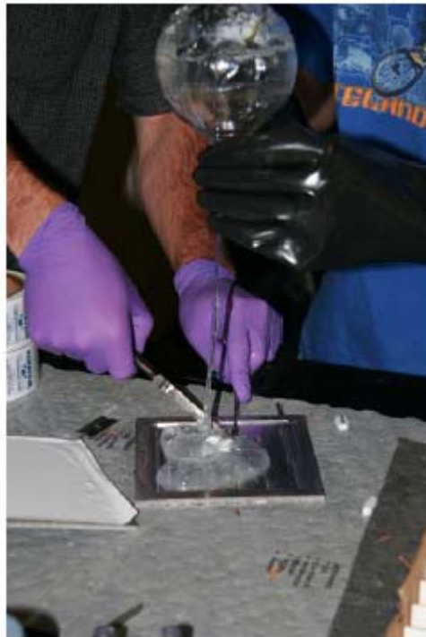
Figure 16: Dissolved UHMWPE pressed into a sheet
