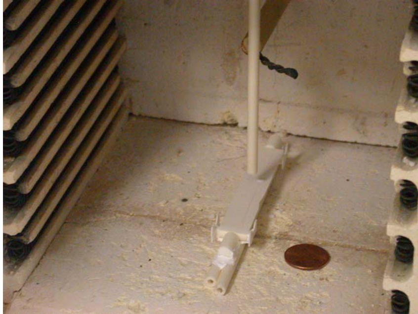
Figure 51. A picture showing the high temperature 3-point bend test fixture inside the box furnace. The 3" x 0.5" x 125 \mu\text{m} alumina beam is supported on alumina tubes; the load is applied from the top via the guided alumina pushrod. A penny is shown at the right for scale.
