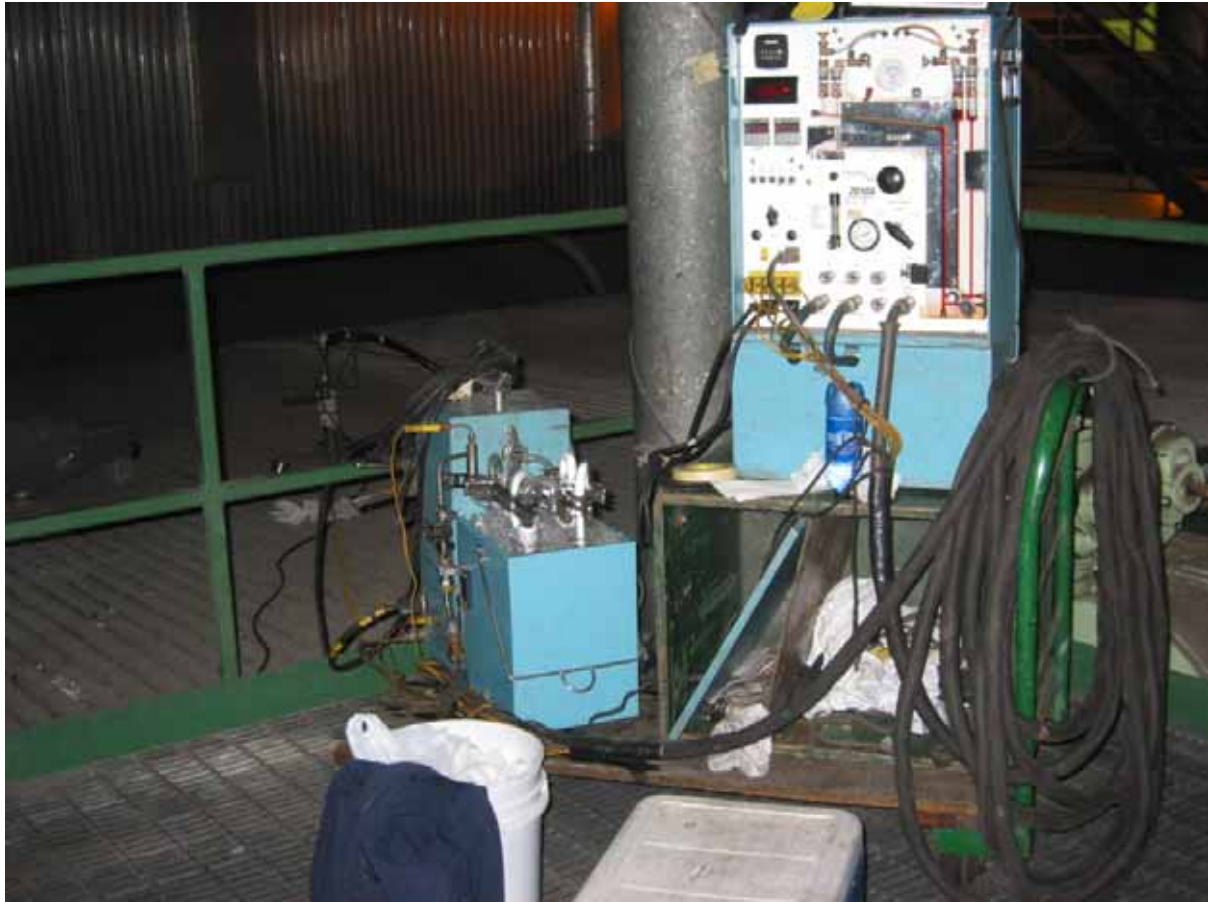
Figure 6. FGD inlet probe (in background), sampling train, and meter box
