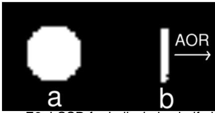
Figure E2. LCSR for helical plus half-circle pinhole-collimator orbit. Transaxial (a) and sagittal (b) slices through the LCSR are shown. The volume is nearly cylindrical, except for defects at the ends (b, bottom), where the valid volume depends on the initial angle of acquisition, and except for binning effects. The axial translation of the orbit is 1.28~cm, which corresponds to two bins. The volume is three bins wide axially due to edge effects and centering.
