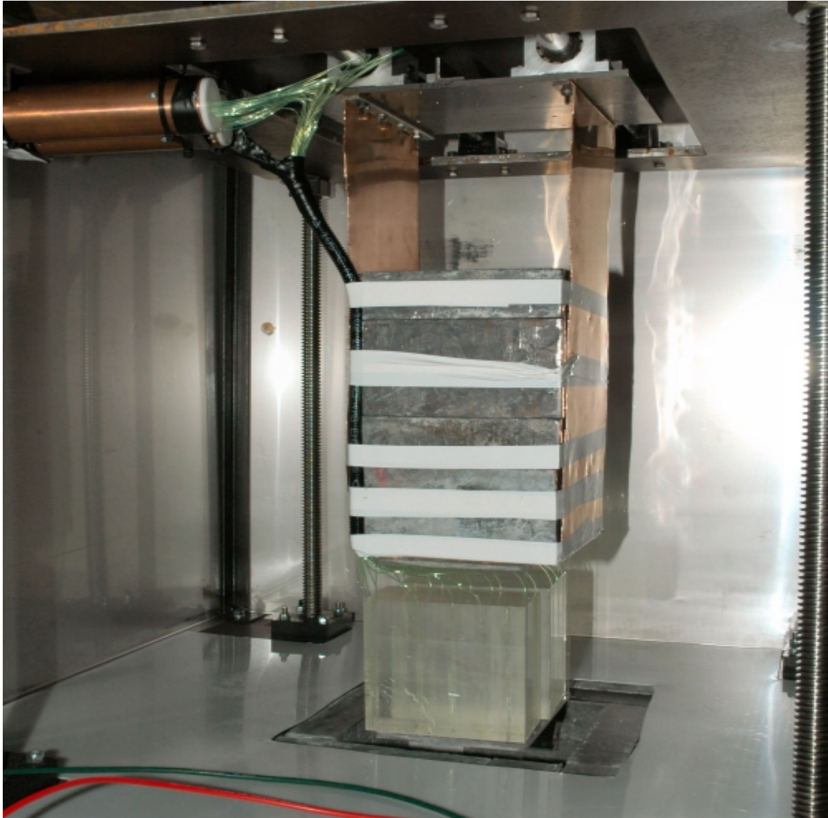
Figure 4 - Plastic scintillation detector (6"x 6"x6") with wavelength shifting fibers and photomultiplier tubes (housed in copper shielding tubes at the upper left)
