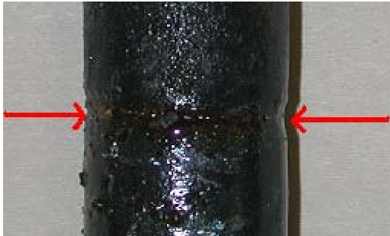
Figure 5. External surface of a Monofrax K-3 refractory rod after partial immersion and rotation at 9.2 rpm in the IP30LAW-C iron phosphate melt at 1100°C for 7 days. The melt line indicated by red arrows was hardly visible.
