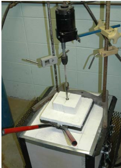
Figure 2. External view of the dynamic corrosion test apparatus.
