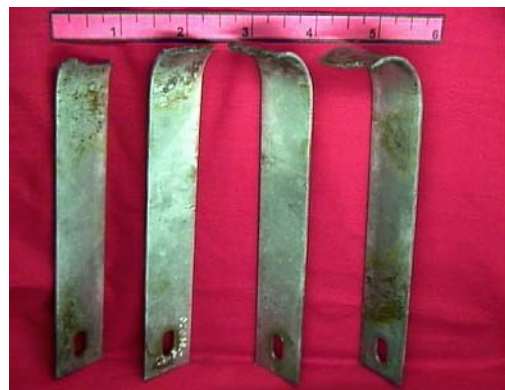
Figure 6. Cleaned stress corrosion specimen.
