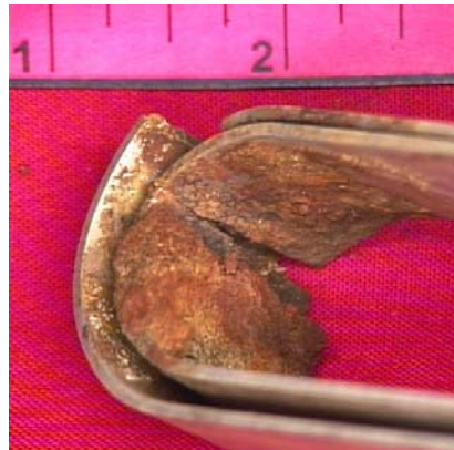
Figure 5. Fractured stress corrosion specimen.
