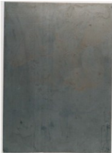
Figure 3. Annealed Type 316 plate with little visible corrosion.
