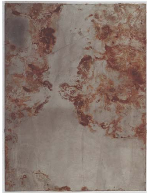
Figure 4. Corroded surface of Type 301 plate.
