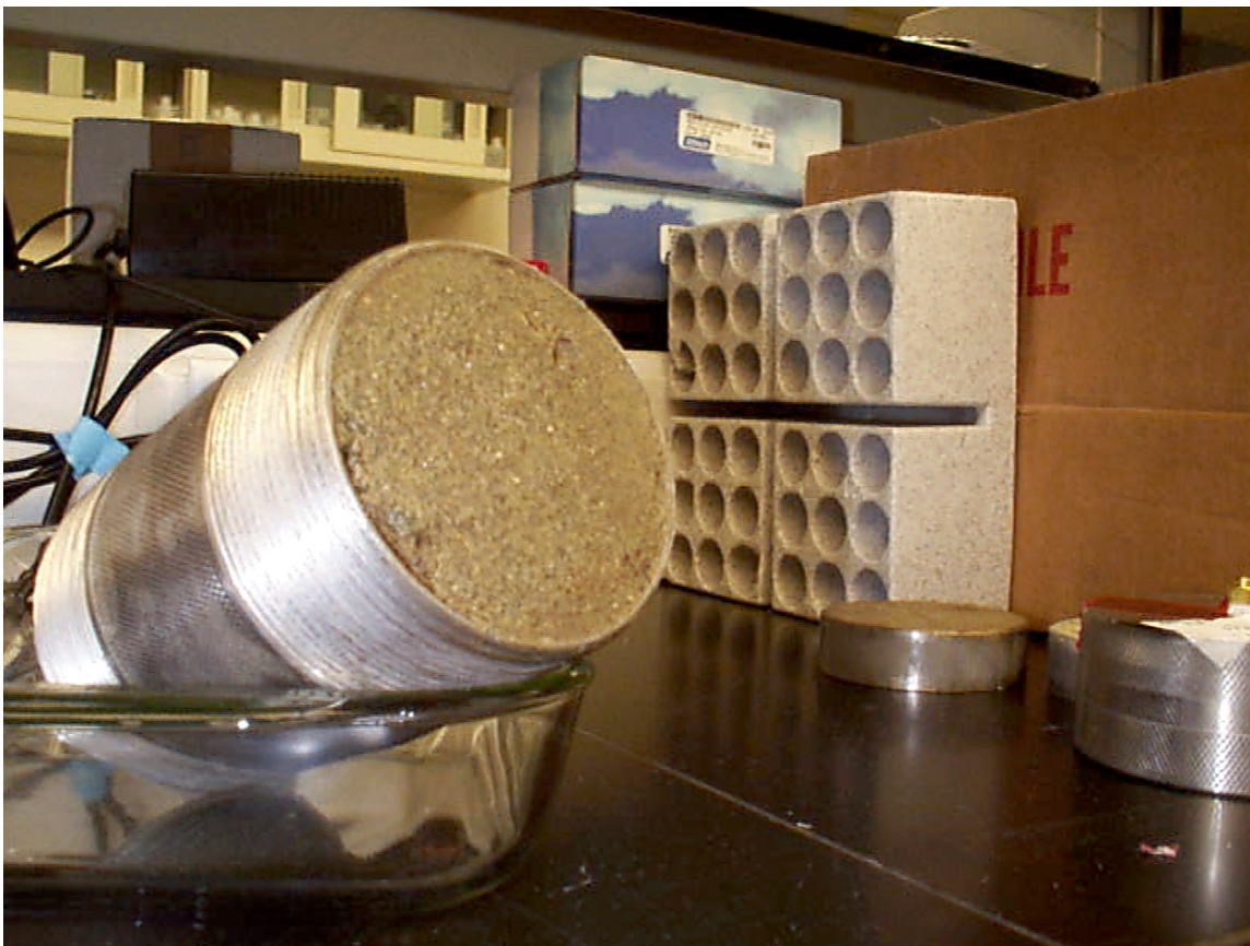
Figure 1. Sediment from the Ringold Formation (364-366 ft depth below ground surface) at the DOE's Hanford Site is shown within the sample collector.
