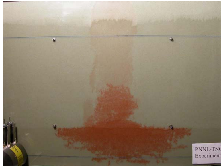
Fig. 4. Photograph of LNAPL distribution 45 days after the rise. The lower and upper blue lines indicate the location of the initial and final water table.
