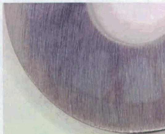
**Figure 9.** Specimen JE3297 After CPP in 0.225 m  $\text{MgCl}_2$  + 22.5 m  $\text{Ca}(\text{NO}_3)_2$  at  $145^\circ\text{C}$
