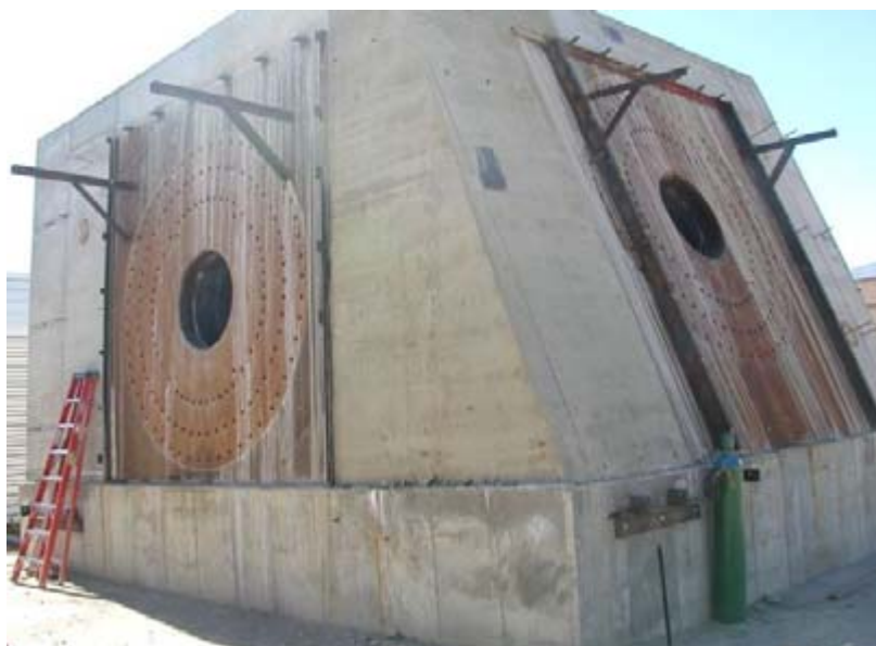
Figure 4: 50-m blade test stand outside of the NWTC blade test facility
