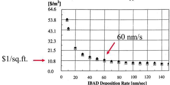
Maximum Production Volumes for Available Equipment Film Thickness: Al<sub>2</sub>O<sub>3</sub> 4 μm, Cu&Ag 200 nm
