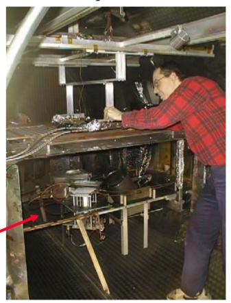
Evaporators and ion source located at bottom of chamber
