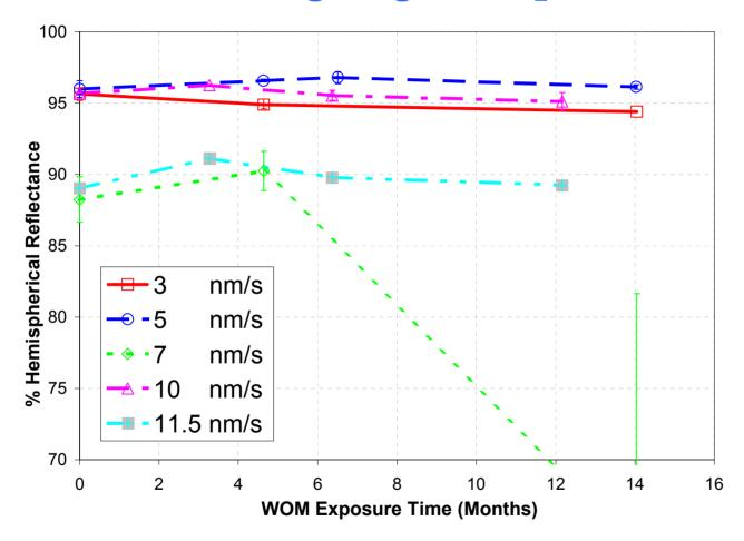
Samples with 10x increase in deposition rate still durable.
