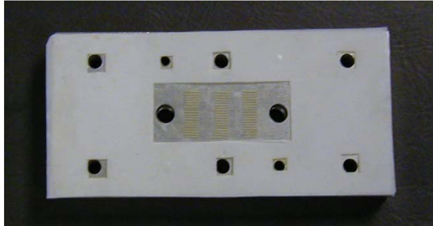
Figure 3.4. Teflon mold and three sensors.
