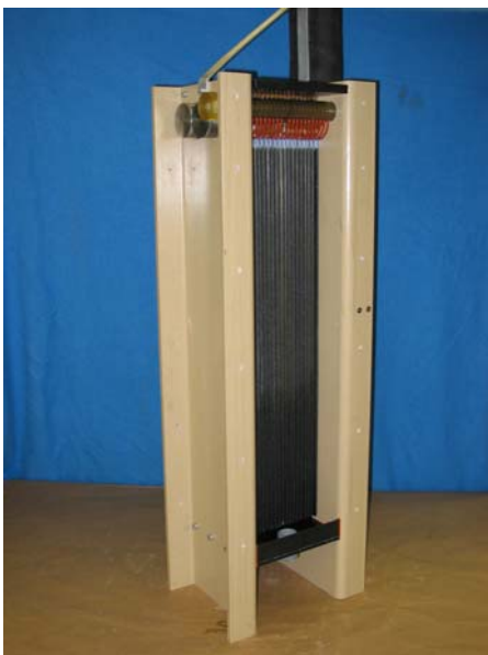
Figure 5 – A low-flow scavenging-air regenerator
