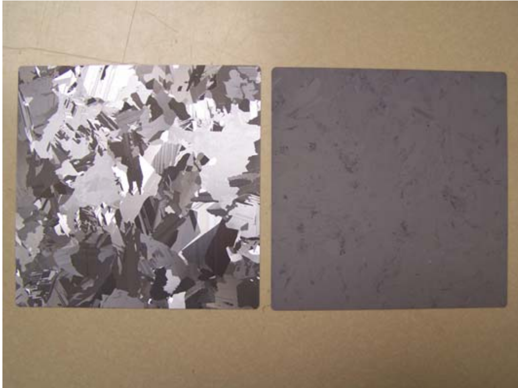
Figure 21: NaOH versus Iso-Chemical Texture on Multicrystalline Silicon
