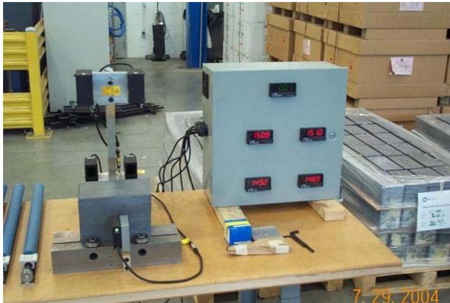
Figure 35: Brick Measurement System
