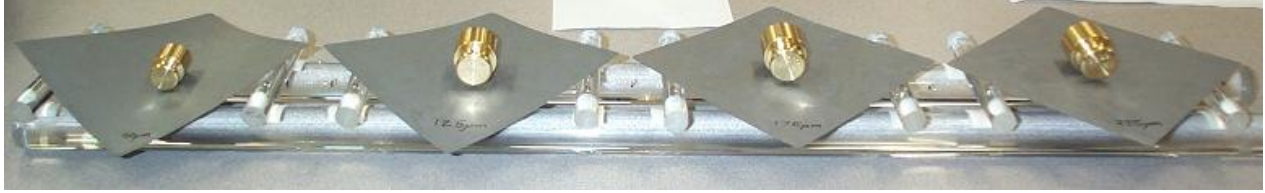
Figure 7: Different Thickness Wafers under Stress (wafer thickness from left to right: 90 \mu\text{m} - 125 \mu\text{m} - 175 \mu\text{m} - 225 \mu\text{m} ) (Weight from left to right: 50 g - 100 g - 100 g - 100 g)
