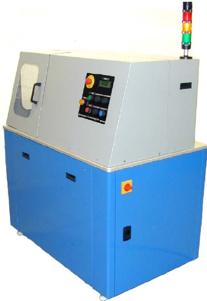
Figure 6a. ATI Wet Wafer Cassetting Machine
