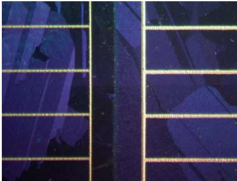
Figure 25: Hot Melt (left) and Screen Print (right) Metallization
