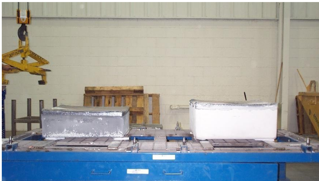
Figure 2: Standard Ingot and Larger 320 kg Ingot
