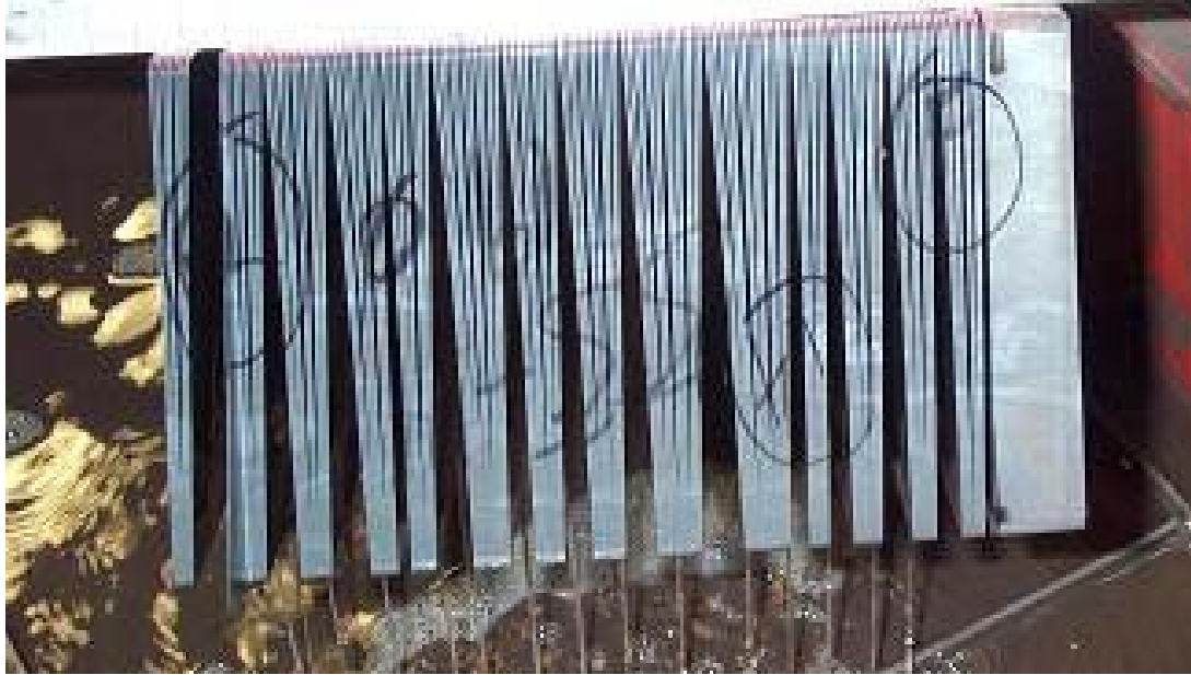
Figure 4: Thin Wafer Comb as it came off of the Wire Saw
