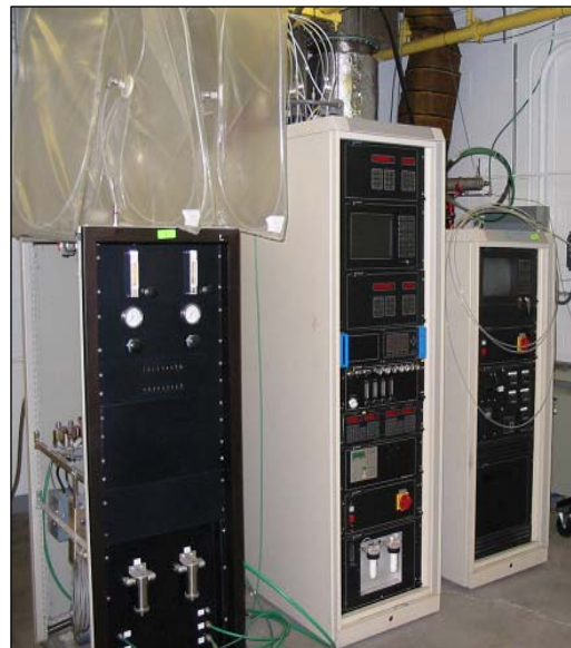
Figure 4. Pierburg Emissions Bench
