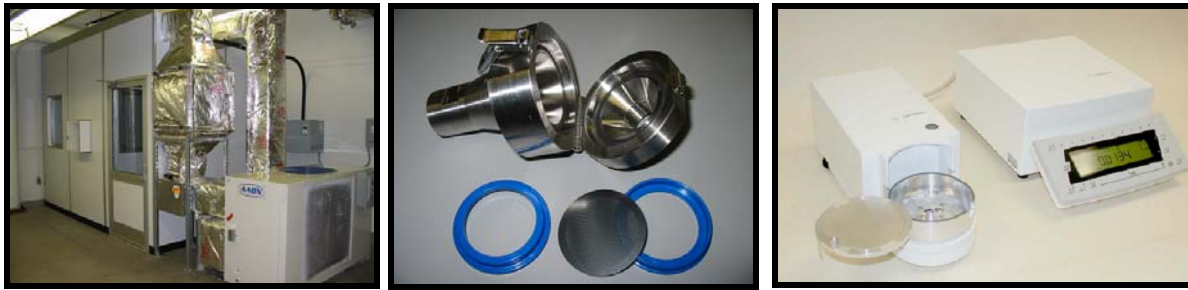
Figure 5. Class 1000 Clean Room, Filter Housing, and Microbalance
