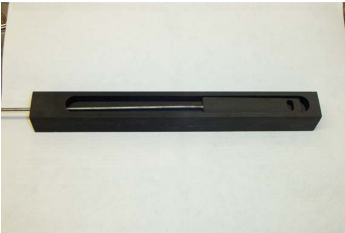
Figure 5: Sliding boat of the new sliding-boat reactor.
