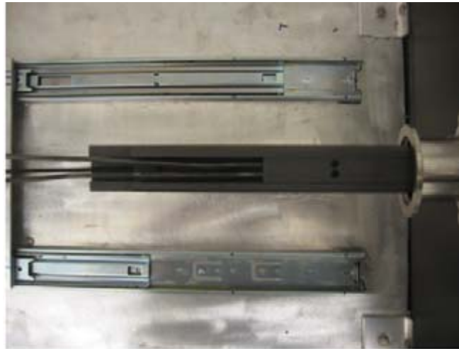
Figure 13: Modified sliding boat mechanism with two thermocouples and the linkage for the linear motion manipulation of the underlying substrates.
