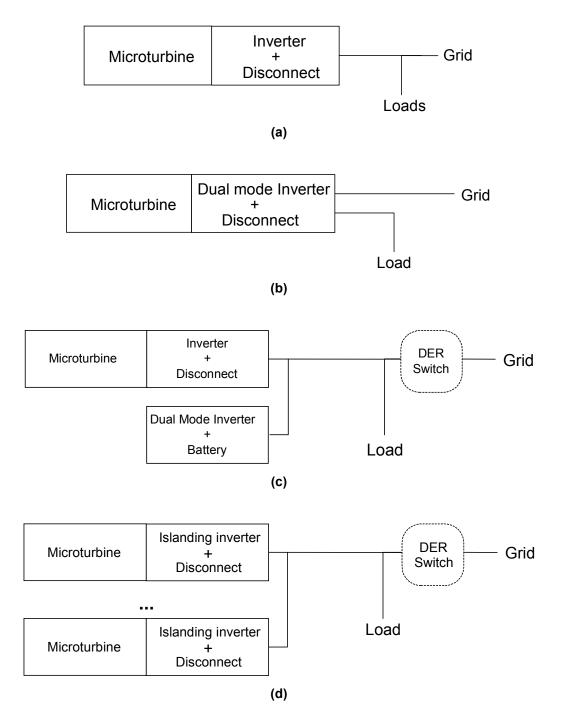
Figure 4. DG architecture with dispatchable sources: (a) Grid parallel configuration (b) Dual mode inverter with grid parallel and stand alone capability and do not require additional DER Switch (c) Upgrade of grid parallel configuration to provide backup (d) Multiple DG configuration that requires additional DER switch.
