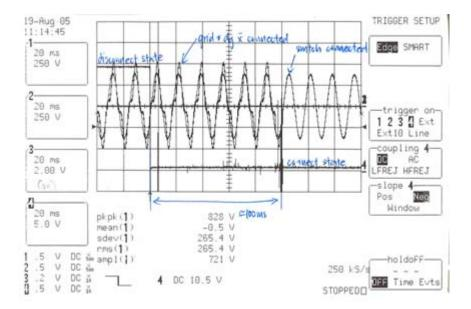
Figure 22. Waveforms that indicate switch connection transition
