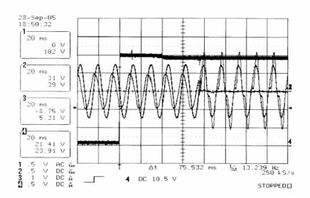
Figure 24. Waveforms that indicate switch disconnection transition
