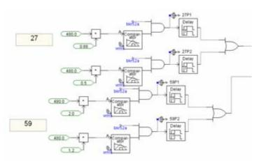
Figure 2. Logic controllers for under- and overvoltage trip functions
