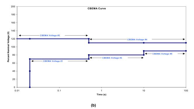
Figure 29. CBEMA curve specification defined in controller
