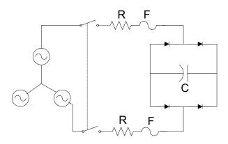
Figure 17. Clamp capacitor pre-charge circuit
