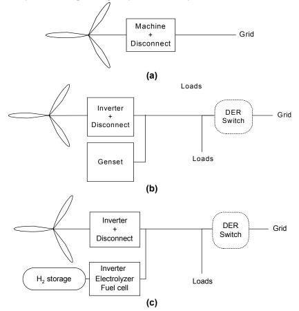
Figure 3. Architecture for wind DG and hybrid wind systems
