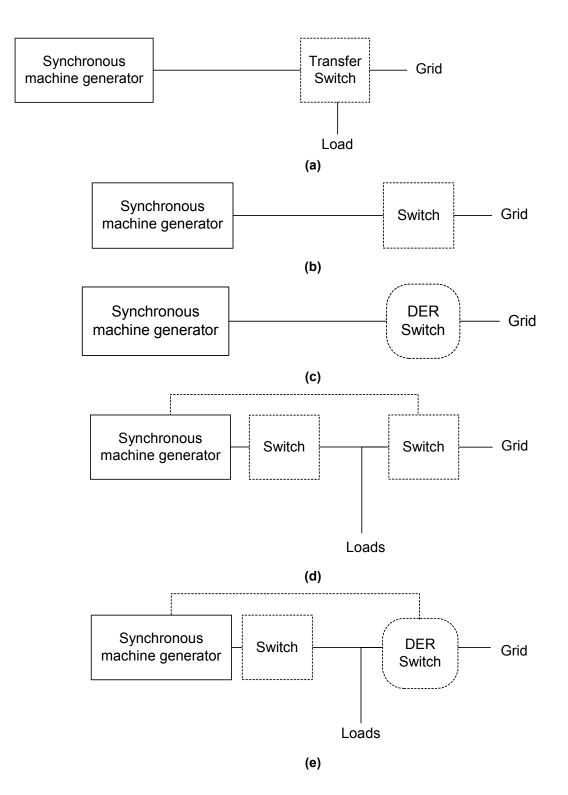
Figure 5. Interconnection architecture with synchronous machine generators: (a) Gensets with transfer switches (b) Traditional grid interconnection configuration (c) Grid interconnection configuration using DER Switch (d) Traditional grid interconnection configuration with islanding capability (e) Grid interconnection configuration with islanding capability using DER Switch.
