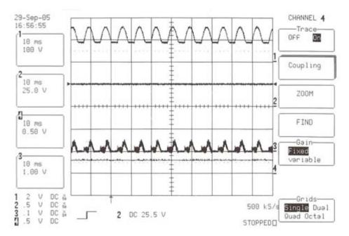
Figure 21. Voltage and current steady-state response of the input and output terminals of the 24Vdc power supply
