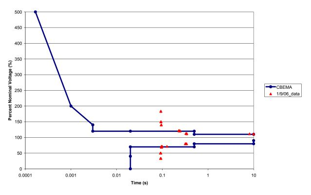
Figure 2. Power Quality test results
