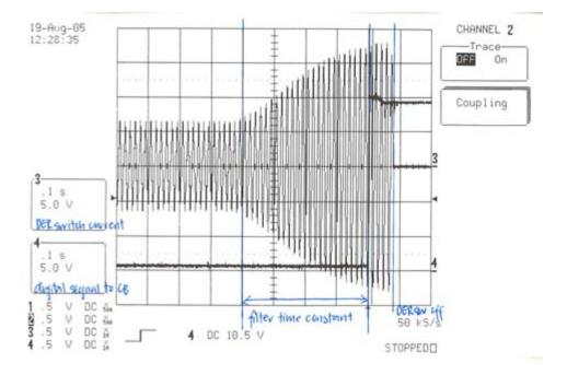
Figure 25. Switch response to a large undervoltage event
