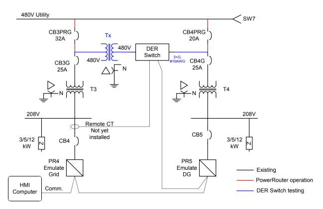
Figure 19. NPS's setup for testing the DER Switch in the Waitsfield test facility
