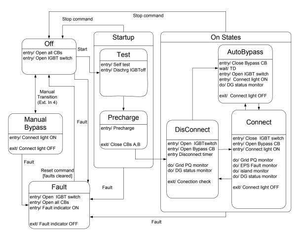
Figure 10. State diagram for the DER Switch
