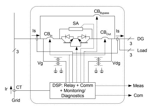
Figure 11. One-line schematic of the DER Switch showing sensor locations
