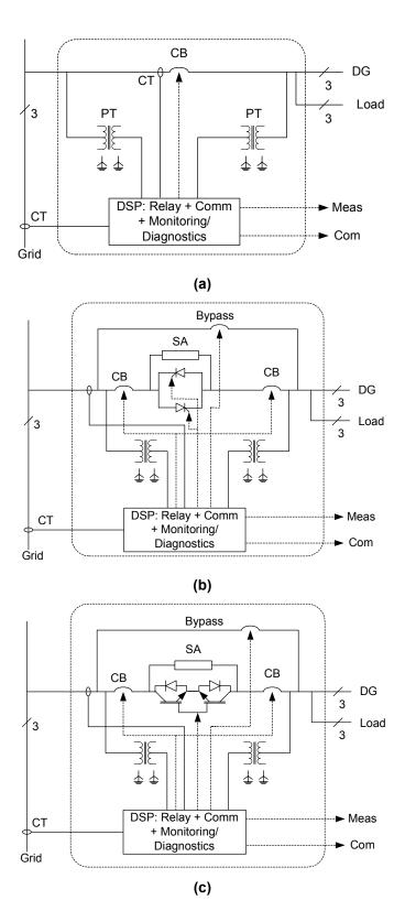
Figure 8. A typical circuit configuration of a DER Switch using (a) CBs, (b) SCRs, and (c) IGBTs
