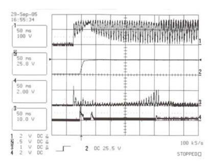
Figure 20. Voltage and current start-up transient response of the input and output terminals of the 24 Vdc power supply
