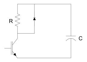
Figure 18. Clamp discharge circuit
