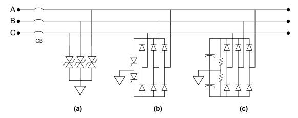
Figure 16. Voltage suppression topologies for three phase applications: (a) Voltage surge suppressors, (b) crowbar circuits, (c) clamp snubber circuits
