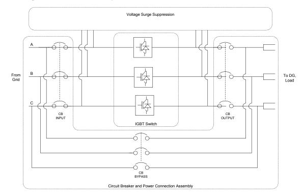
Figure 14. Circuit configuration of the DER switch
