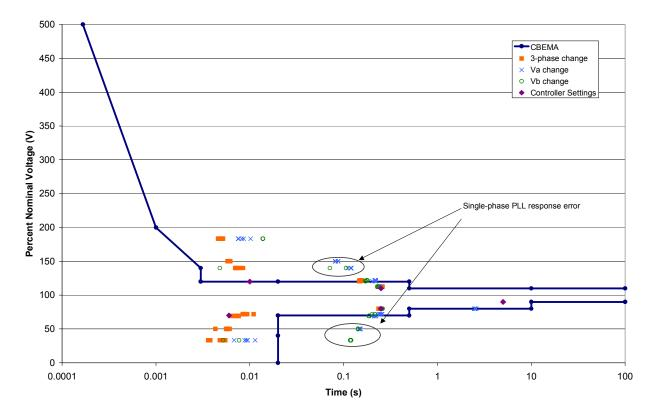
Figure 32. CBEMA curve test performed at NREL
