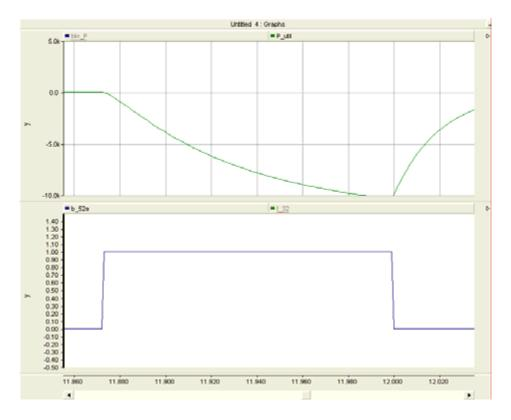
Figure 10. Anti-islanding (via 5 kW reverse power)
