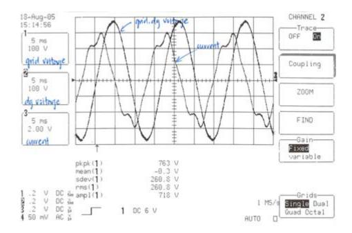
Figure 23. Voltage and current waveforms after switch closing
