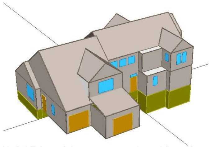
Figure 13. DOE-2 model geometry as viewed from the northeast with shading surfaces hidden, generated using eQuest
