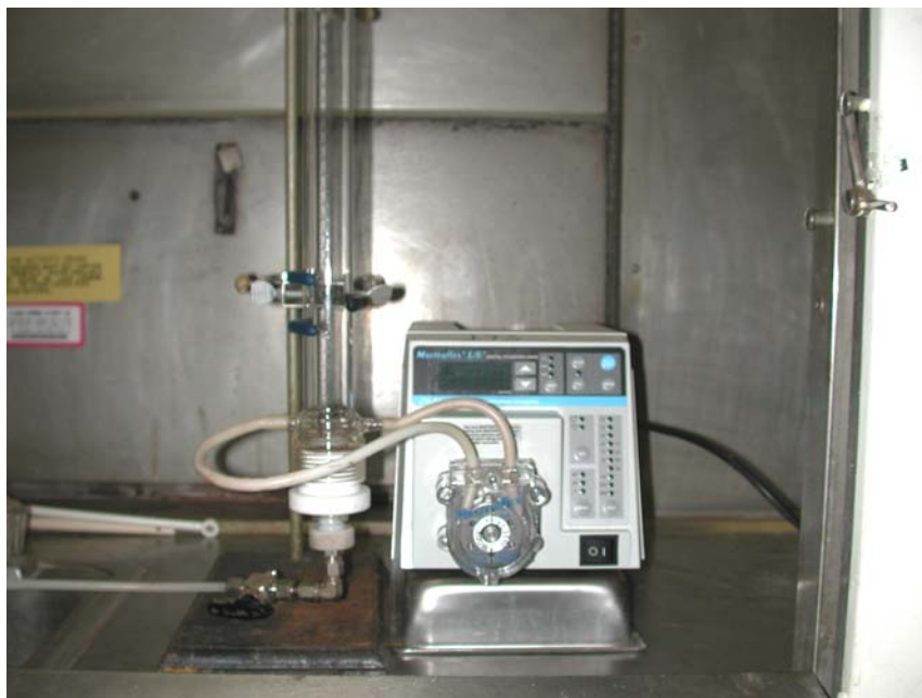
Figure 19. Foam Column with Recirculation Loop
