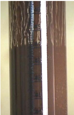
Oxidative Leach of High Cr Simulant at 4 hours after start of reaction, Flux = 2.2 \text{ ft}^3/\text{min}/\text{ft}^2 Foam ht. = 44 cm Foaminess = 1065%
