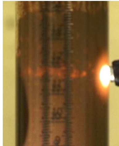
Oxidative Leach of High Cr Simulant with 350 ppm Antifoam at 6 hours after start of reaction. Flux = 2.2 \text{ ft}^3/\text{min}/\text{ft}^2 Foam ht. = 11.5 cm Foaminess = 203%
