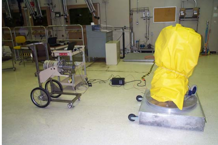
Figure 1 Temporary Assay Facility with wrapped heater box on turntable.
