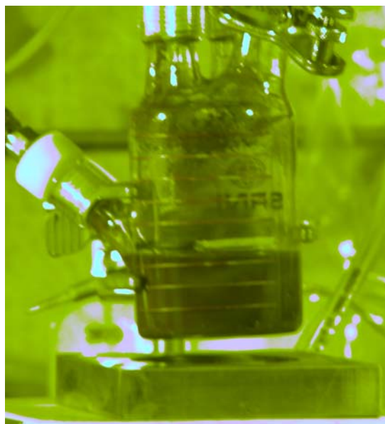
Figure 4. Evaporator Vessel at End of Run
