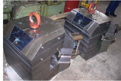
Figure 3: NESTOR bending magnet after reconstruction.
