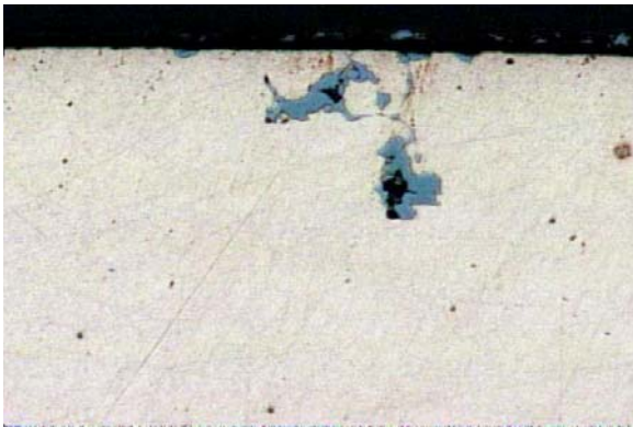
500X, 50-day test, 50-ppm, 40/20°C, with intergranular attack. See right for etched condition.
