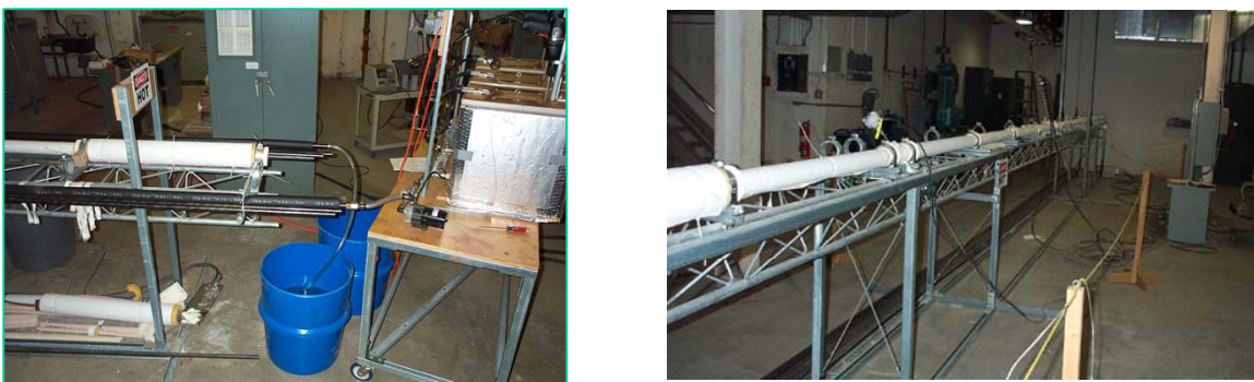
Figure 1. The modified state-of-the-art apparatus for lining 40-ft.-long heat exchanger tubes using impedance heating system.
