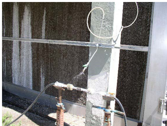
Figure 5. OMP coatings exposed to brine spray at Mammoth.
