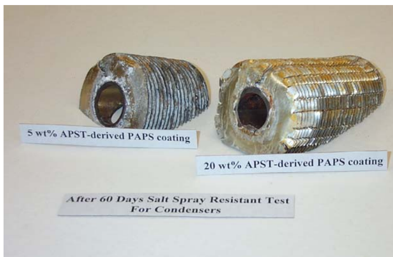
Figure 2. Appearance of the condensers coated with 5wt% and 20wt% APST-derived PAPS after a 60-day salt-spray resistant test: Corroded condenser (left) and non-corroded one (right).
